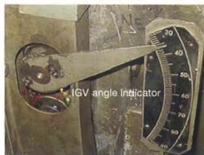
8-10. Inlet guide vanes control the flow of air entering the compressor. IGV angle indicator is shown alongside the vane actuator
