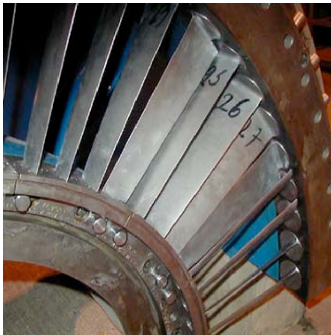
Fig. 1: Typical Variable Inlet Guide Vanes (VIGV) showing inner bushing blocks and dowels
