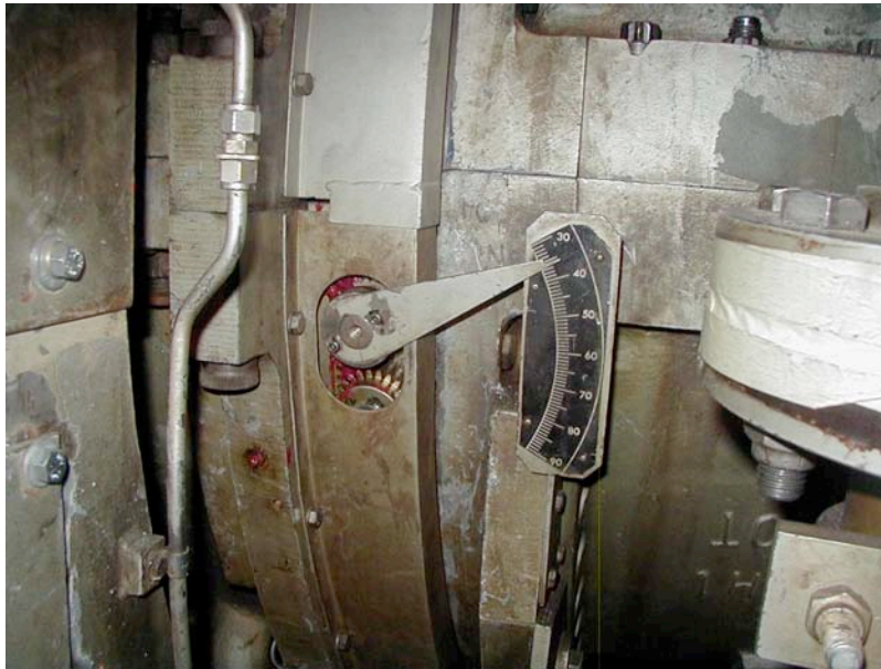
IGV angular position indicator and pointer
