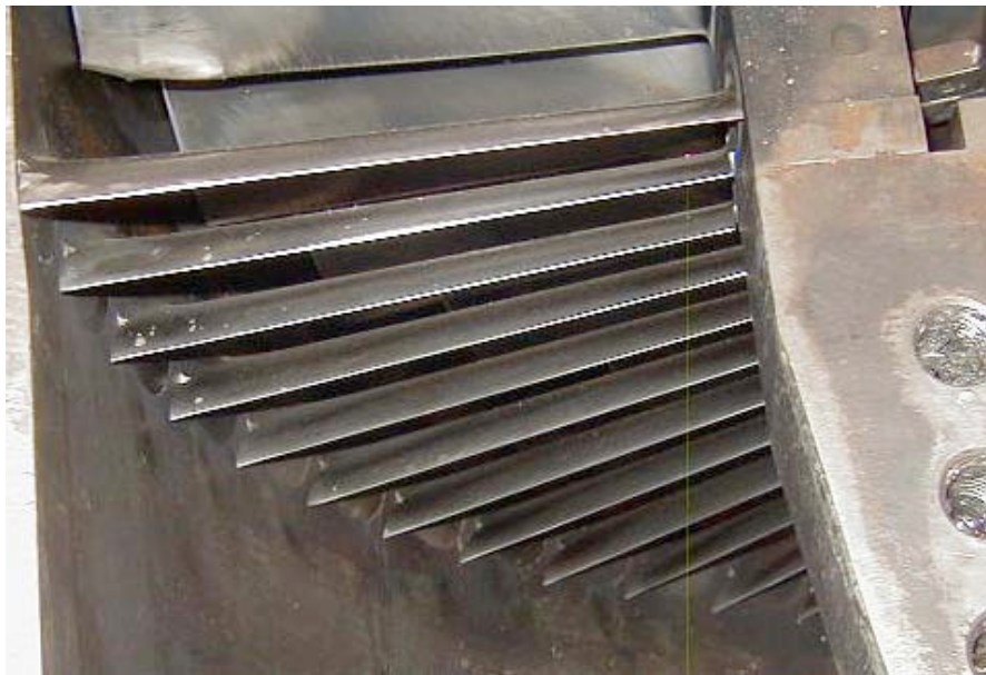
Leading edge of VIGV with compressor rotor blades (damaged) in background
