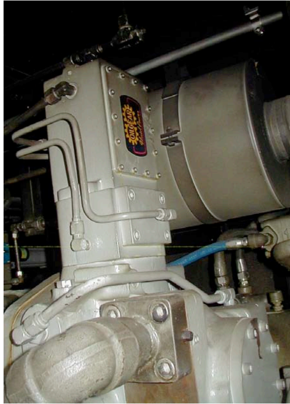
Fig. 4: VCO Servo Actuator for OilGear Fuel Pump
