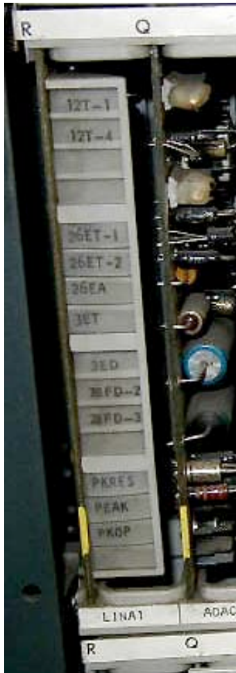
Fig. 2: LINA card with 4 unused lamps (Row 1, Slot R) on a typical Mark I panel
