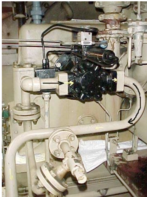
Fig. 1: NY Airbrake Fuel Pump showing fuel flow
