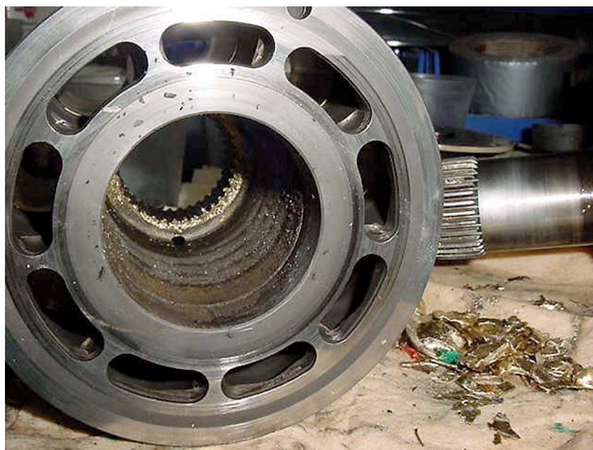
Fig. 3: Failed NY Airbrake Fuel Pump with copper debris
