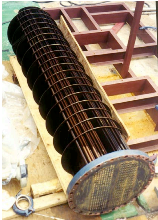
Fig. 4: Heat exchanger tube bundle being prepared for shipment
