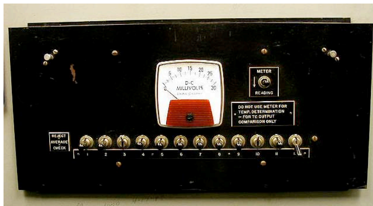
Fig. 3: Thermocouple Averaging Cabinet
