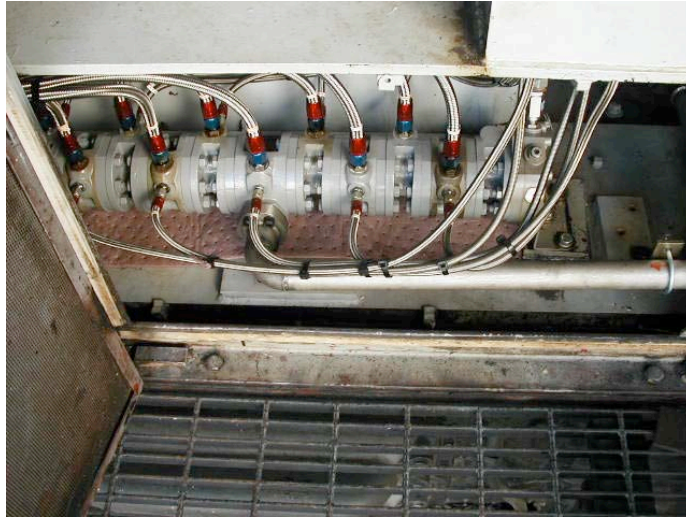
Fig. 2: Flow divider tubing using high-pressure braided hosing
