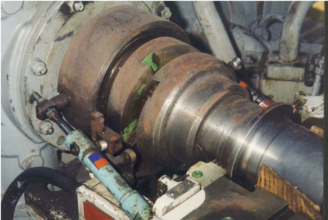
Fig. 4: Clutch Position Limit Switch 33CS (Red nameplate on device shown at bottom left)
