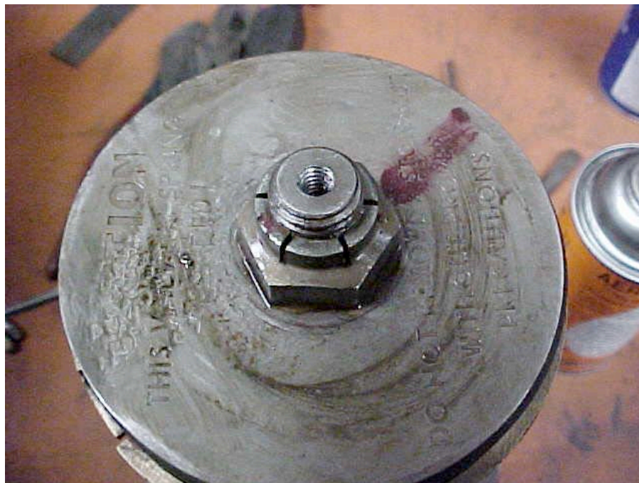
Fig. 4: Top of valve stem is drilled and tapped
