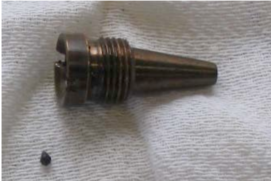
Fig. 4: Venturi unscrewed and removed atop gear box. Debris or clog is also shown
