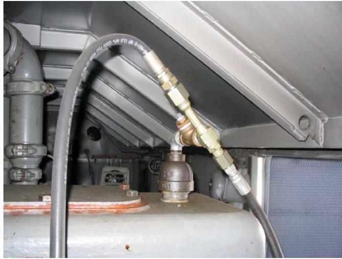
Fig. 2: Air lines going to and from venturi
