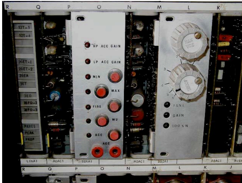
Fig. 5: Manual VCE “Gag” on the SSZA Card at slot location 1L1M.
