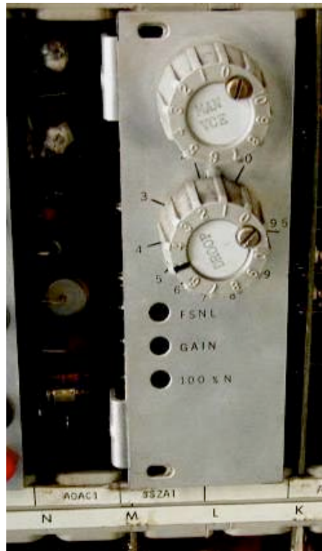
Fig. 1: SSZA card with MAN VCE Resistor
