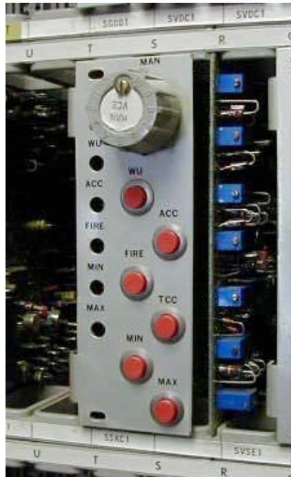
Fig. 2: SSKC card with MAN VCE resistor
