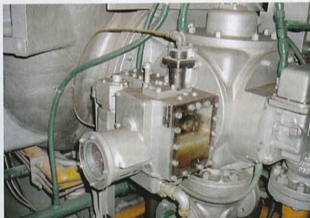
only unit certainly is less complicated than that for the dual-fuel machine in Fig 3 6. Fuel regulator is driven off the accessory gearbox
