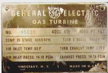
4. Nameplate for GE gas turbine S/N 95095 provides design data. Additional information of interest: Air flow to the compressor at rated conditions is 98 lb/sec, temperature of compressed air flowing to the combustors is 500F, combustion gas enters the turbine at 81.7 psia/1400F
