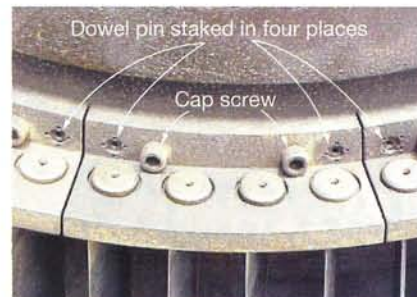
6. Each ring segment is retained by two staked dowels and two cap screws
