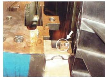
10. Rub-ring groove runs around the lower half of the bellmouth from horizontal joint to horizontal joint
