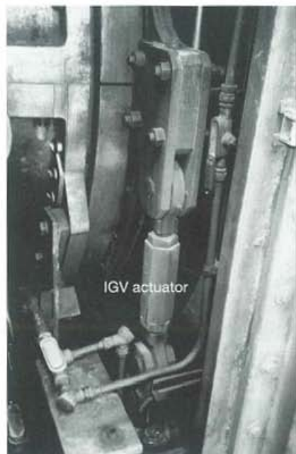
8-10. Inlet guide vanes control the flow of air entering the compressor. IGV angle indicator is shown alongside the vane actuator
