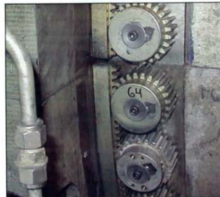
Figure 4: Operators should always consider IGV inspection and upgrade every outage. A high-flow IGV yields more output
