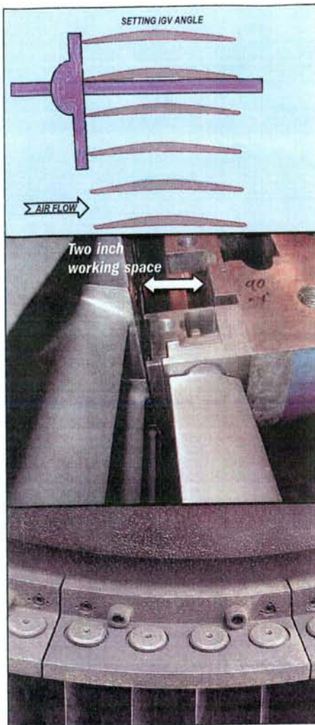
Clockwise from top Figure 6: New-style IGVs have a small fillet that prevents crack formation Figure 7: Parts in IGV assembly Figure 8: Inlet bellmouth and IGVs Figure 9: Jacking bolt modification added to bellmouth Figure 10: IGVs and support blocks Figure 11: Support block bolted to inlet bellmouth Figure 12: Removing the lower half IGVs is difficult because the working space is only 2 inches Figure 13: Protractor used to set vane angle
