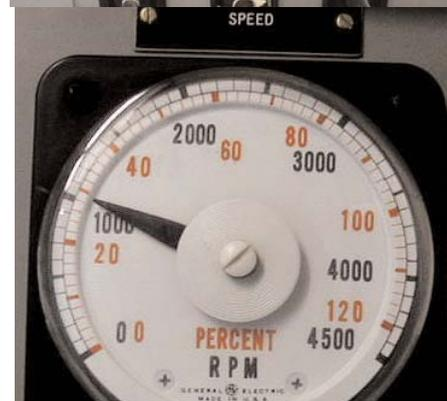
Figure 4: Turbine compressor speed indicator (rpm and percent)
