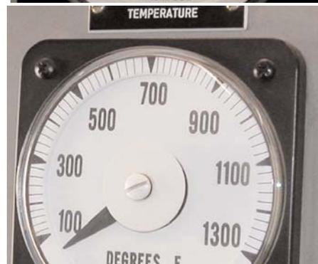
Figure 5: Average exhaust temperature, TXA
